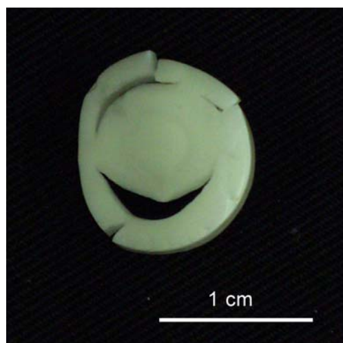
Fig. 5 Shrinking rupture of the PDEAMG-30 immersed in water at 40 °C
